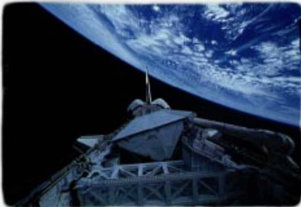
Fig. 3 – Shuttle Imaging Radar –C (SIR-C) deployed in the open payload bay of STS-68
